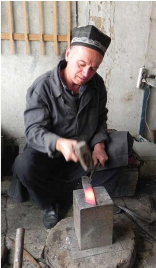
Knife making starts by choosing a piece of suitable metal and identifying type of knife to be made. Than chosen metal is 3 to 4 times put into fire and hammered for the blade to be prepared. After the blade is given desired shape it is than polished by rough and soft sand. More the blade is fired sharper and stronger it becomes. The final polishing is done by using leather or an animal skin with finer hair.
